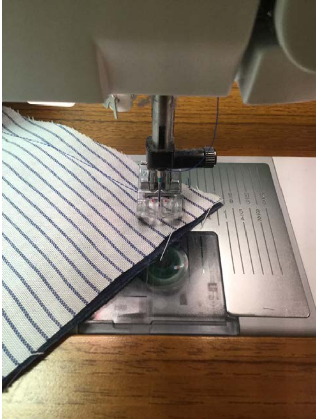
Figure 1: Fabric turned 45 degrees to take one stitch when turning the corner.
